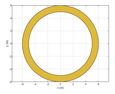
Mesh the ring at a maximum edge length of 1 m.
