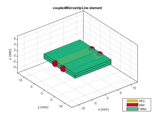
Plot the current and charge distribution on the transmission line. current(coupledmicrostripline, 4e9)
