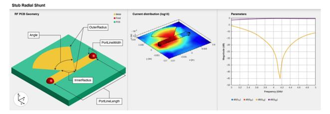
Radial stubs provide broadly resonant RF short circuits by introducing the short at a concentrated point. When cascaded with high-impedance quarter-wavelength transmission lines, radial stubs provide an effectively decoupled network for microwave amplifiers and other active components.
