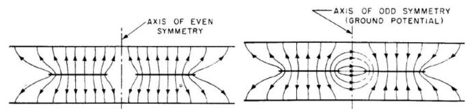
The figure shows transverse field distributions for two fundamental transverse electro-magnetic (TEM) modes. These modes exists on a pair of parallel conducting strips between parallel ground planes.
