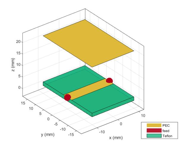
Calculate the S-parameters over the 10 frequencies from 1-5 GHz.
