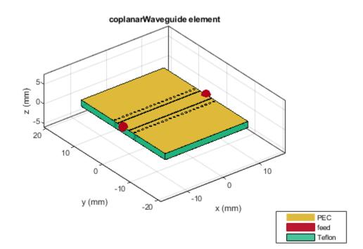
Calculate the S-parameters of the waveguide from 1-10 GHz.
