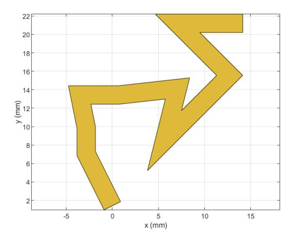
Mesh the custom line trace at a maximum edge length of 1 m. mesh(customLine,MaxEdgeLength=1)
