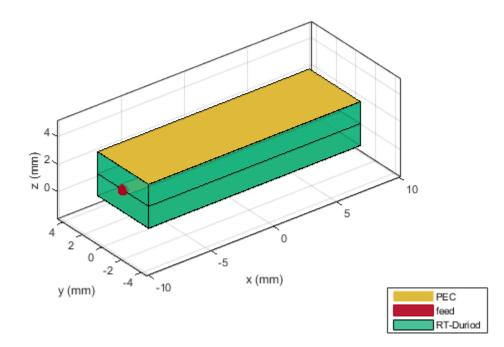
Plot the s-parameters of this transmission line.
