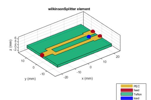
Calculate and plot the S-parameters of the splitter at 3 GHz.
