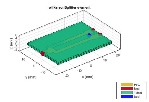
Plot the charge and current on this splitter at 3 GHz.
