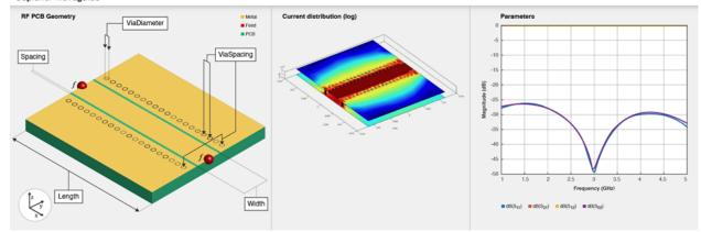
To analyze the behavioral model of a coplanar waveguide transmission line, set the Behavioral property in the sparameters object function to true or 1.
