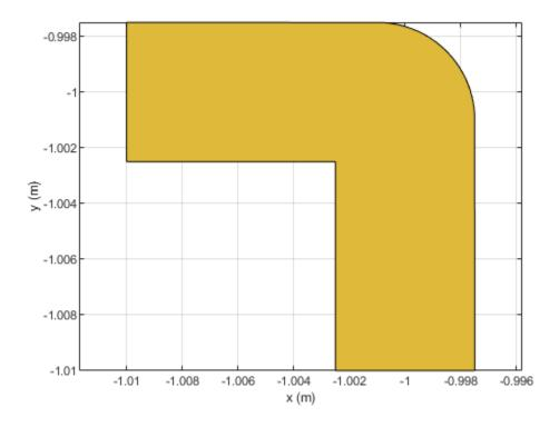
Subtract the offset bend from the default bend and display the result.
