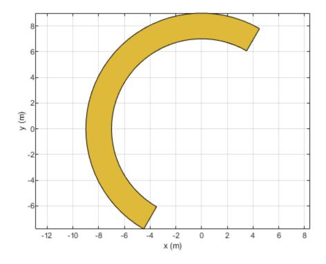
Mesh the curved shape at a maximum edge length of 1 m. mesh(curved,MaxEdgeLength=1)
