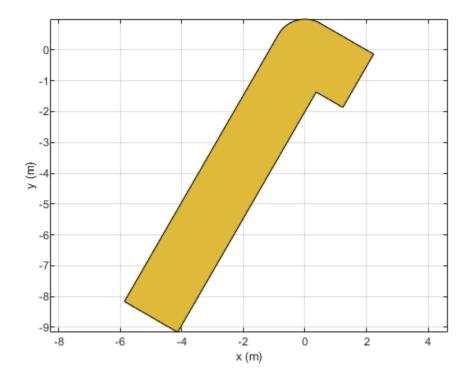
Mesh the curved bend shape at a maximum edge length of 1 m.
