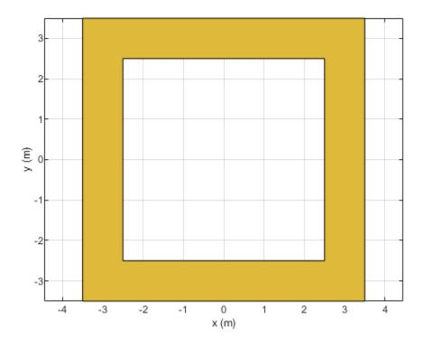
Mesh the square ring at a maximum edge length of 1 m. mesh(ring,MaxEdgeLength=1)
