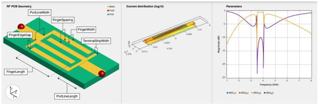
A two-port series IDC with microstrip form feeder lines supports single and multiple dielectrics. It is a coplanar structure consisting of multiple comb electrodes or intersecting fingers with spaces between the fingers. An IDC can have identical port line lengths and widths on either sides.
