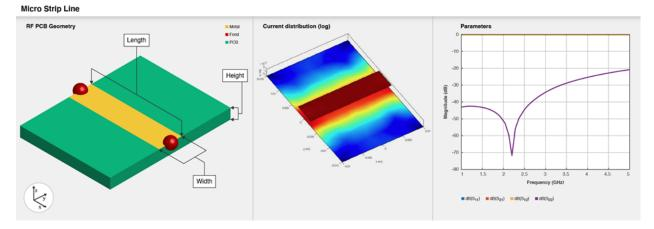
To analyze the behavioral model for a microstrip transmission line, set the Behavioral property in the sparameters function to true or 1.
