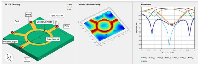
The rat-race coupler is used as a splitter with a phase shift. When given two inputs, the coupler can create sum and difference ports for added and subtracted power. It also acts as an interface between transmitters and receivers for integrating with an antenna and in building circuits with complex functionality like a comparator with sum and difference ports.
