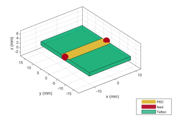
Calculate S-parameters over 10 frequencies from 1-5 GHz.
