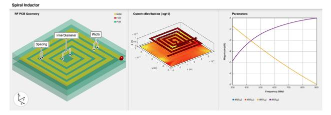
To analyze the behavioral model of a spiral inductor, set the Behavioral property in the sparameters function to true or 1.
