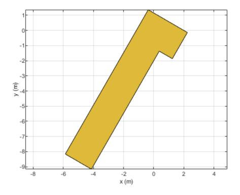
Mesh the right-angle bend shape at a maximum edge length of 1 m. mesh(bend,MaxEdgeLength=1)
