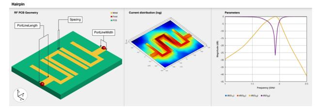
Hairpin filters are easy to fabricate. Design these filters at different frequencies by changing the rolloffs and the ripple factors. You can control the bandwidth of the filter by varying the filter order, width, and the distance between the coupled lines. There are two types of hairpin filters based on the feed: tapped-line input hairpin filters and coupled-line input hairpin filters.
