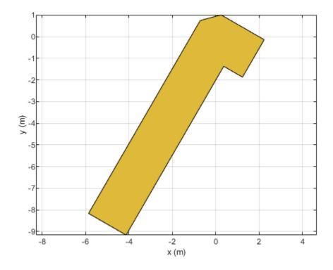
Mesh the mitered bend shape at a maximum edge length of 1 m. mesh(bend,MaxEdgeLength=1)
